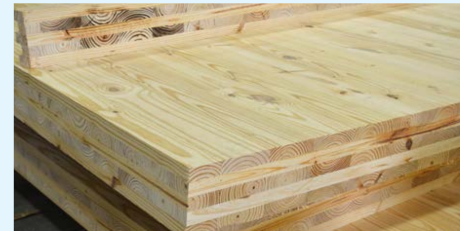
The CFWE actively promotes the use of cross-laminated timber, or CLT, a mass timber product made of southern pine and other soft woods abundantly found in the region. Using CLT has numerous benefits economically and environmentally, thereby showing promise for many industries, including developers and contractors, architects and engineers, as well as foresters and landowners.
