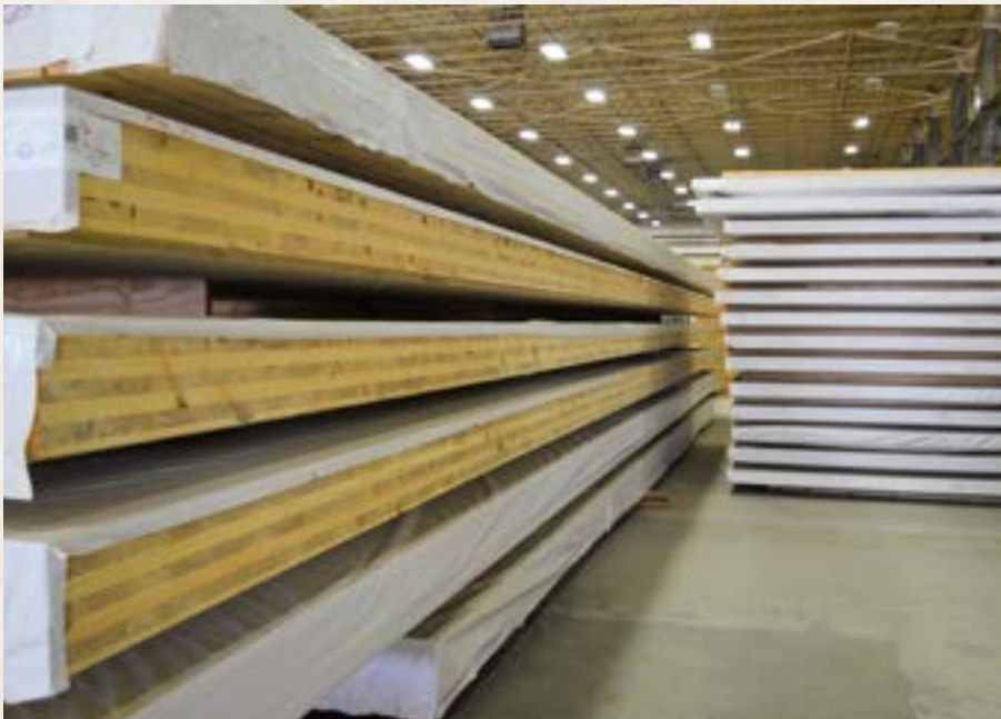
Attendees visited the SmartLam North America cross-laminated timber, or CLT, manufacturing plant in Dothan, where participants learned how CLT is engineered and prefabricated to a building project’s exact specifications and requirements. Shown are fabricated CLT panels prepared for shipment.
