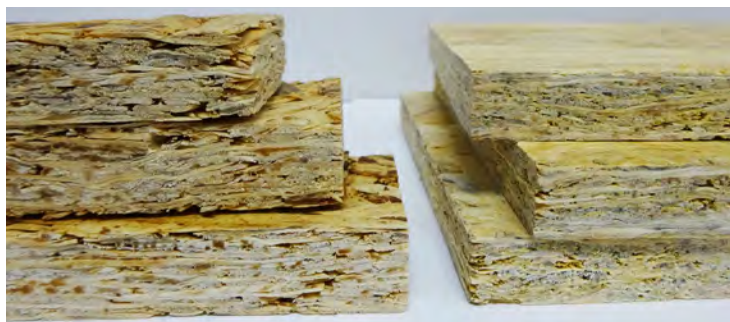
The addition of water to oriented strand board (OSB) is problematic because it causes irreversible swelling and this difficulty could be compounded if the wet adhesive strength/bond is not adequate. Wet OSB, left, and original OS, right, are pictured above.
